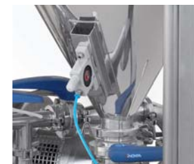
9A802-020: pneumatic vibrator. (button in the control panel to stop/start the vibrator).
