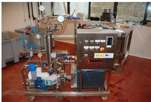
**Figure 1.** Alcoholic strength reduction system.
