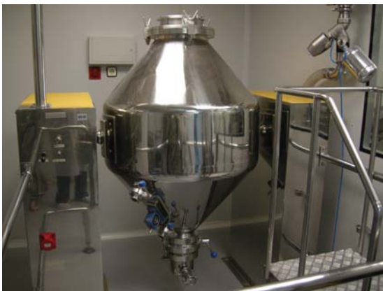
Double cone blender with an automatic loading/discharge system
