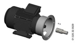
3. Hold the pump cover (03) on the lantern (04) with the hand and gauge the assembly position according to the distance A.
