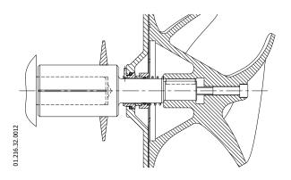
ATTENTION! When installing the new seal, use soapy water when fitting the different parts and gaskets to allow them to slide better; apply to the stationary as well as the rotating parts.
