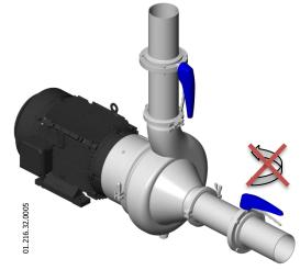
Reduce the flow rate and the electrical power consumed by the motor:
