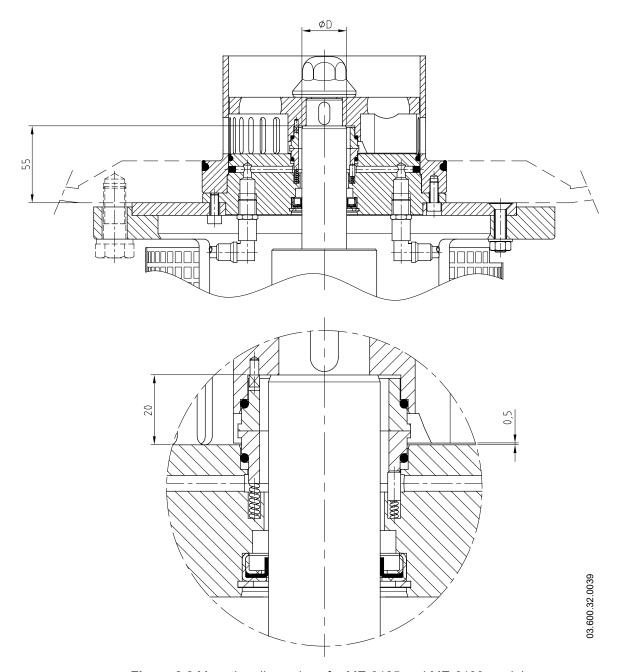
Figure 8.2 Mounting dimensions for ME-6125 and ME-6130 models
