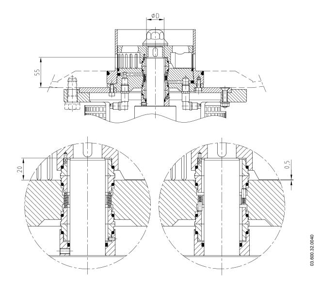
**Figure 8.4** Spring detail to ME-6125 and ME-6130 mixers
